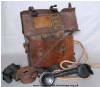
(left) DIII Telephone. Used by signallers in World War I, we found it to be an ideal linesman's telephone.
